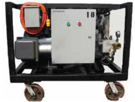
60 HP/ 60GPM Pump
